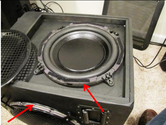
Extra spacers for cone excursion at LAB 12C & PRs (LAB12C excursion too high for full grill)
