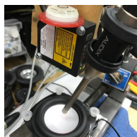
Test set-up for peak linear displacement measurement
